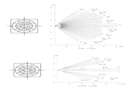
Fig 8.Top and Side view of each Facet in a PIR Sensor
