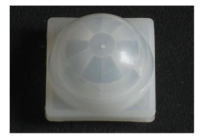
Fig 6. Multi Facet-Sections of Fresnel Lens
