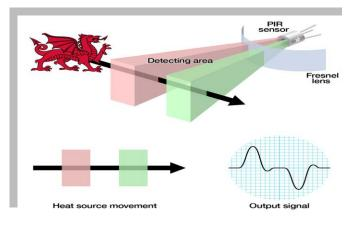
Fig 3 Working of PIR Sensor
