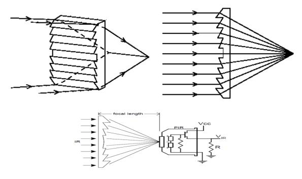
Fig .5 Incident Radiation on Fresnel Lens
